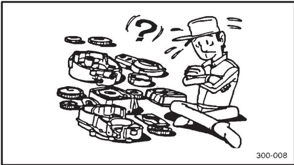
4. When disassembling the machine, always keep mated parts together. This includes gears, cylinders, pistons and other parts that have been "mated" through normal wear. Mated parts must always be reused or replaced as an assembly.
