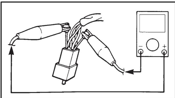
3. Connect and disconnect the connector two or three.
