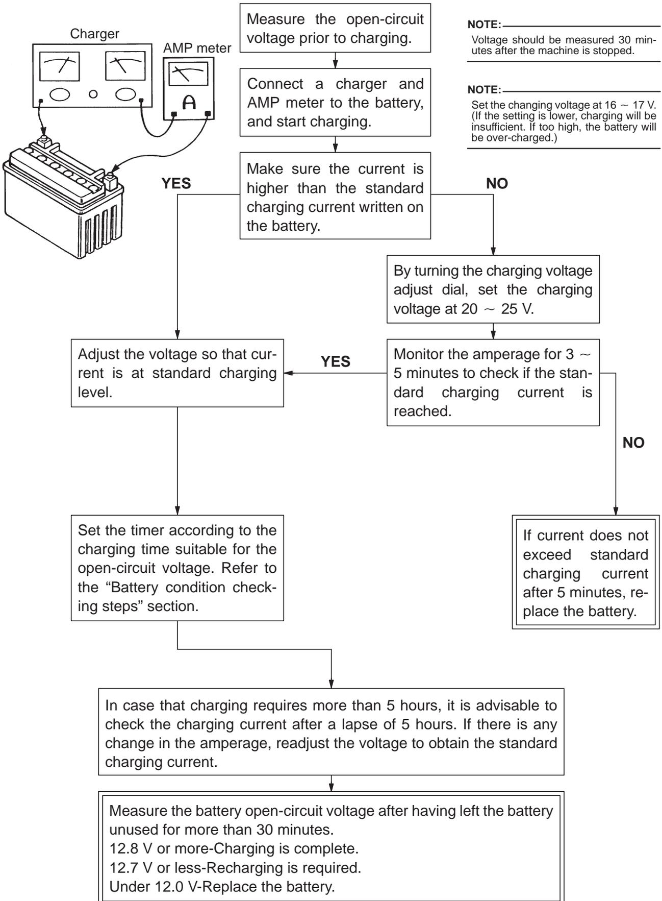
**Charging method using a constant-voltage type charger**
