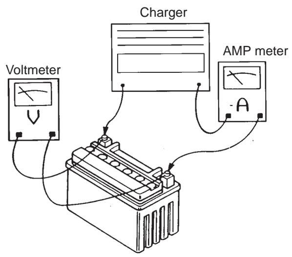
**Charging method using a constant-current type charger**
