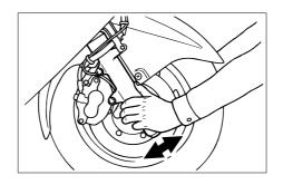
Hold the lower ends of the front fork legs and try to move them forward and backward. If any free play can be felt, have a Yamaha dealer check or repair the steering. EAU01144
