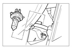
5. Place a new headlight bulb into position, and then secure it with the bulb holder.
