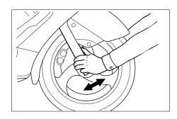
Hold the lower ends of the front fork legs and try to move them forward and backward. If any free play can be felt, have a Yamaha dealer check or repair the steering.
