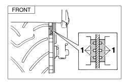
1. Brake pad wear indicator groove (×3)
