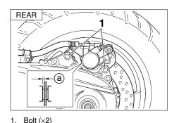
Tightening torque: Brake caliper bolt: 40 Nm (4.0 m·kg)
