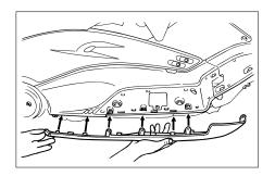
To install the panel Place the panel in the original position, and then install the screws.
