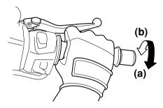
The speed can be adjusted by opening and closing the throttle. To increase the speed, turn the throttle grip in direction (a). To reduce the speed, turn the throttle grip in direction (b).
