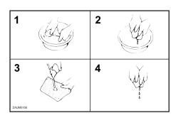
Apply oil of the recommended type to the entire surface of the element, and then squeeze the excess oil out.
