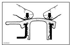
2. To install the 2-stroke engine oil tank cap, push it into the oil tank opening.
